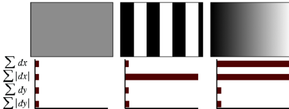
Fig. 3. The descriptor entries of a sub-region represent the nature of the underlying intensity pattern. Left: In case of a homogeneous region, all values are relatively low. Middle: In presence of frequencies in x direction, the value of \sum |dx| is high, but all others remain low. If the intensity is gradually increasing in x direction, both values \sum dx and \sum |dx| are high.
