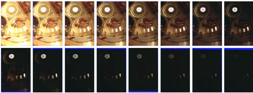
Figure 6: Sixteen photographs of a church taken at 1-stop increments from 30 sec to \frac{1}{1000} sec. The sun is directly behind the rightmost stained glass window, making it especially bright. The blue borders seen in some of the image margins are induced by the image registration process.
