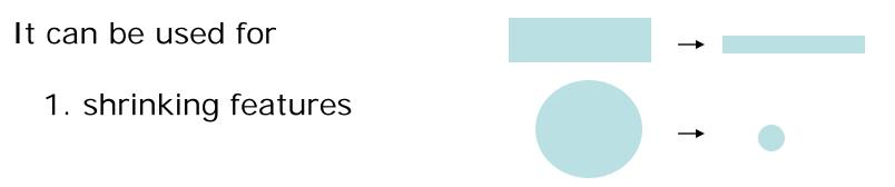
2. Removing bridges, branches and small protrusions
