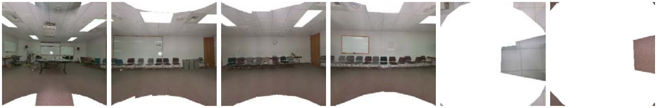
Figure 14: Cubical texture-mapped model of conference room (from 75 images taken with a hand-held digital camera).
