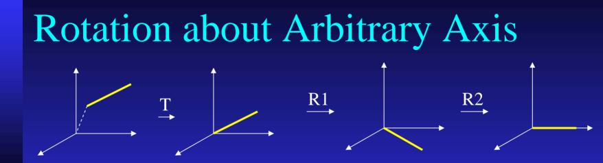
One translation and two rotations to line it up with a major axis. Now rotate it about that axis. Then apply the reverse transformations (R2, R1, T) to move it back.
