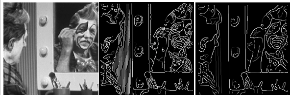
original Canny with \sigma = 1 Canny with \sigma = 2
