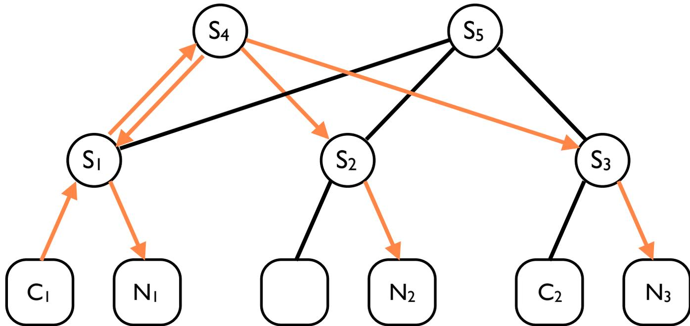
Step 3: Use the same root switch if possible (especially when there are multiple multicast groups)
