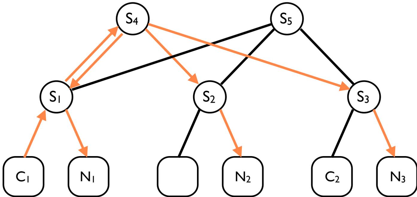
Step 2: Perform in-network replication at the root switch or on the downward path
