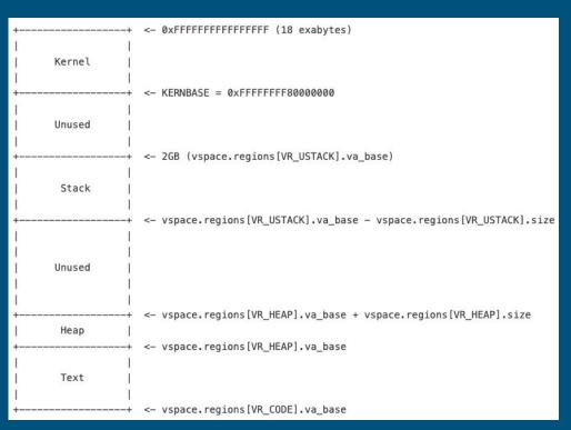
This diagram from memory.md shows the layout of virtual addresses for a process in xk. (The addresses shown on left are <u>virtual</u>).
