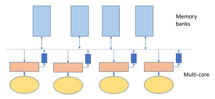
Suppose locations A and B start out with value 0. Core 0 writes 1 to A and then 1 to B, and no one else writes.
