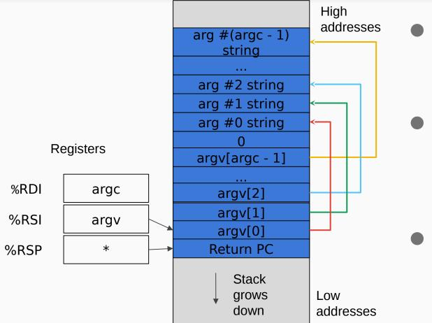
argv is an array of pointers, therefore %RSI points to an array on the stack
