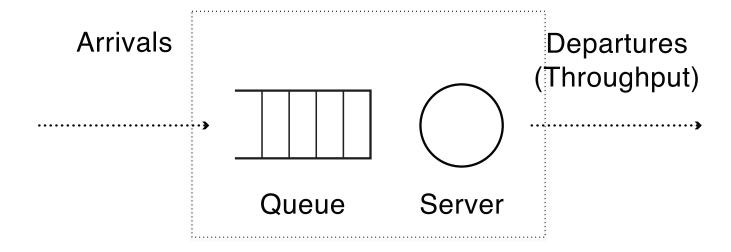
Suppose a system has throughput (X) = 100 tasks/s, average response time (R) = 50 ms/task
