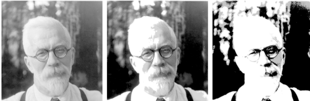
FIGURE 14.9. Sir Ronald A. Fisher (1890 – 1962) was one of the founders of modern day statistics, to whom we owe maximum-likelihood, sufficiency, and many other fundamental concepts. The image on the left is a 1024 \times 1024 grayscale image at 8 bits per pixel. The center image is the result of 2 \times 2 block VQ, using 200 code vectors, with a compression rate of 1.9 bits/pixel. The right image uses only four code vectors, with a compression rate of 0.50 bits/pixel
