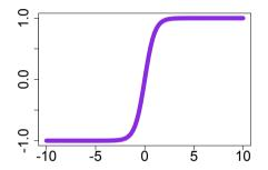
Hyperbolic tangent function,  $\tanh(z) = \frac{e^z - e^{-z}}{e^z + e^{-z}}$ . Generalization: apply elementwise to a vector, so that  $\tanh: \mathbb{R}^k \to (-1, 1)^k$ .
