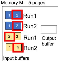
Step 2: Join while merging Output tuples (1,1) (1,1) (1,1) (1,1) (2,2) (2,2)
