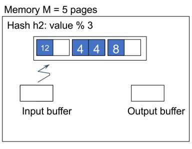
**Step 4:** Scan matching partition of S and probe the hash table
