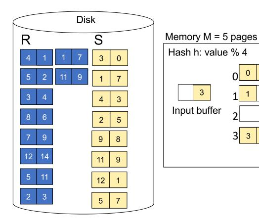
**Step 1:** Read relation S one page at a time and hash into the 4 buckets When a bucket fills up, flush it to disk
