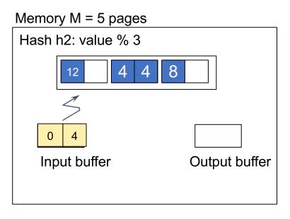
**Step 4:** Scan matching partition of S and probe the hash table
