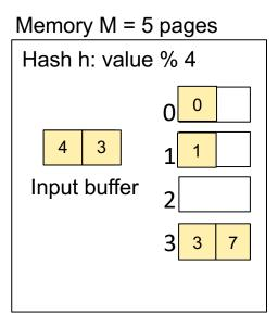
**Step 1:** Read relation S one page at a time and hash into the 4 buckets When a bucket fills up, flush it to disk
