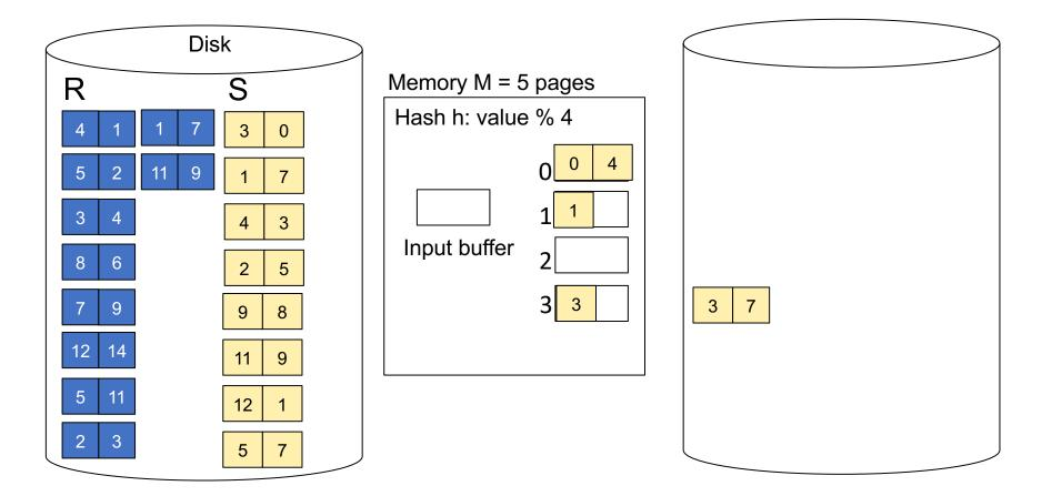
**Step 1:** Read relation S one page at a time and hash into the 4 buckets At the end, we get relation S back on disk split into 4 buckets
