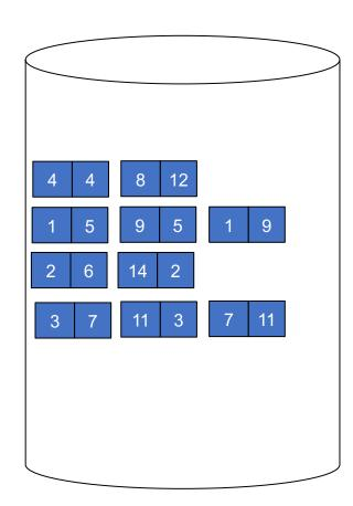
Step 3: Read one partition of R and create hash table in memory using a different hash function
