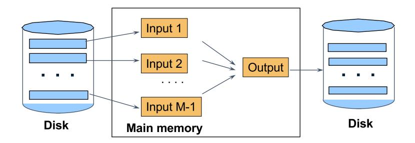
Merging three runs to produce a longer run:
