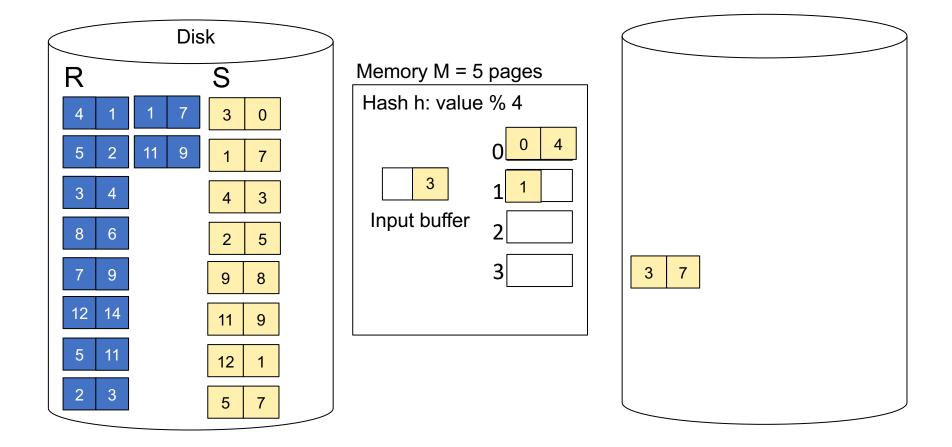
**Step 1:** Read relation S one page at a time and hash into the 4 buckets When a bucket fills up, flush it to disk
