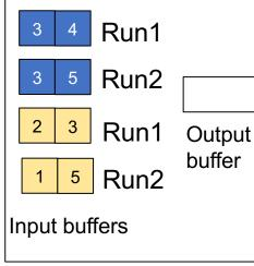
**Step 2:** Join while merging Output tuples
