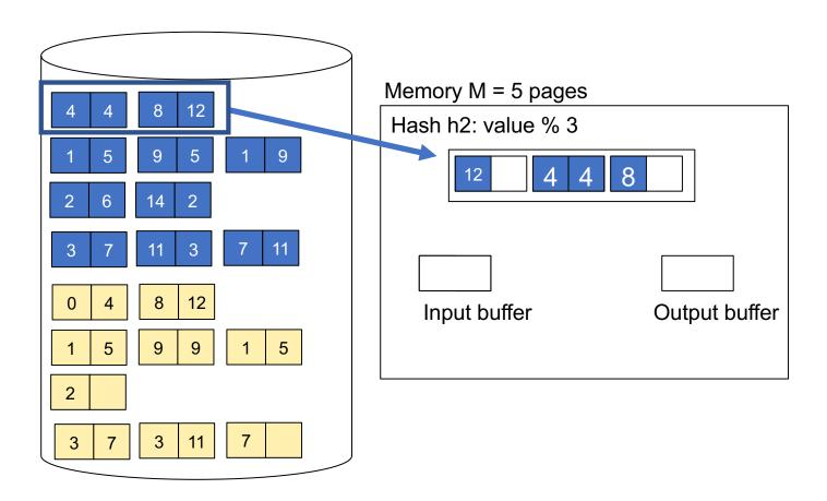
Step 3: Read one partition of R and create hash table in memory using a different hash function
