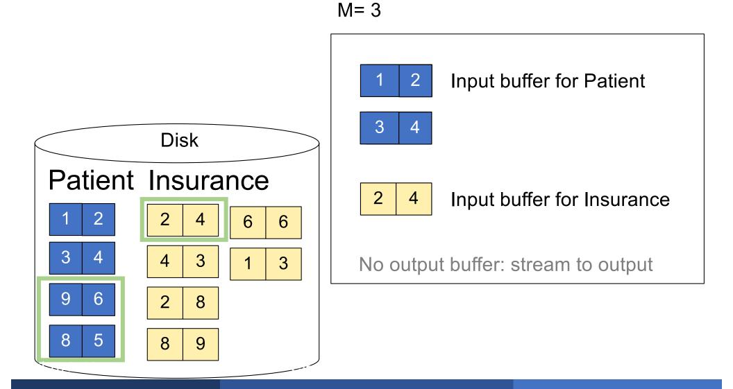
for each group of M-1 pages r in R do for each page of tuples s in S do for all pairs of tuples  $t_1$  in r,  $t_2$  in s if  $t_1$  and  $t_2$  join then output  $(t_1, t_2)$
