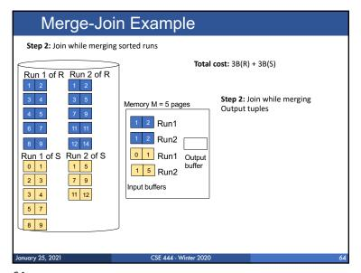
Merge-Join Example Step 2: Join while merging sorted runs Total cost: 3B(R) + 3B(S) Run 1 of R Run 2 of R 1 2 Step 2: Join while merging Memory M = 5 pages Output tuples 1 2 Run1 1 2 Run2 0 1 Run1 Output Run 1 of S Run 2 of S 0 1 1 5 1 5 Run2 2 3 7 9 Input buffers 3 4 11 12 5 7 8 9 January 25, 2021 CSE 444 - Winter 2020
