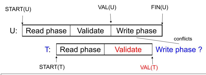
IF  $WS(T) \cap WS(U)$  and FIN(U) > VAL(T)(U has validated and U has not finished before T validates) Then ROLLBACK(T)
