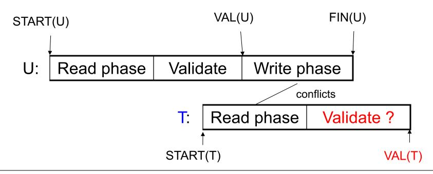
IF  $RS(T) \cap WS(U)$  and FIN(U) > START(T)(U has validated and U has not finished before T begun) Then ROLLBACK(T)
