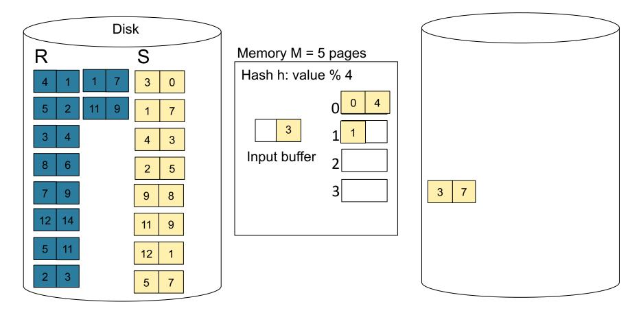
**Step 1:** Read relation S one page at a time and hash into the 4 buckets When a bucket fills up, flush it to disk
