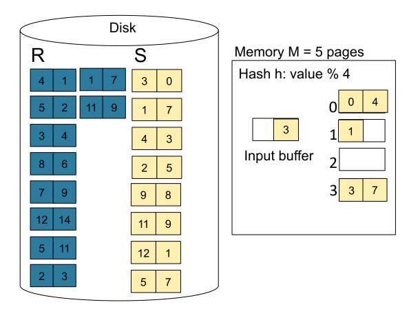
**Step 1:** Read relation S one page at a time and hash into the 4 buckets When a bucket fills up, flush it to disk
