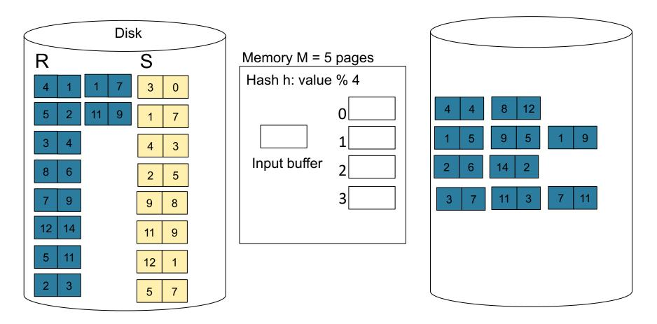
Step 3: Read one partition of R and create hash table in memory using a different hash function
