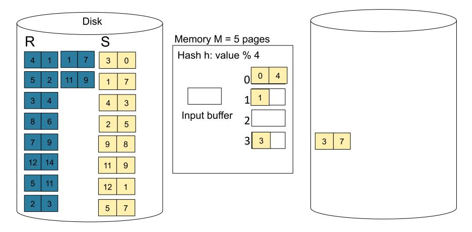
**Step 1:** Read relation S one page at a time and hash into the 4 buckets At the end, we get relation S back on disk split into 4 buckets
