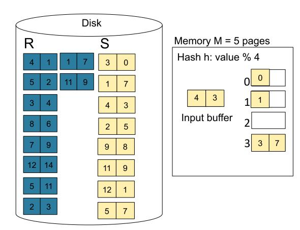
**Step 1:** Read relation S one page at a time and hash into the 4 buckets When a bucket fills up, flush it to disk
