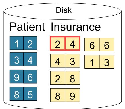
Memory M = 21 pages Hash h: pid % 5 5 3 Output buffer Input buffer Write to disk or pass to next operator 22
