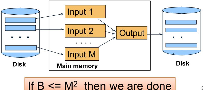
• Merging three runs to produce a longer run:
