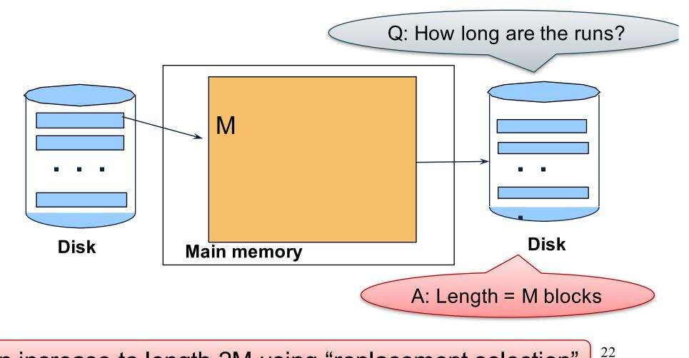
Can increase to length 2M using "replacement selection"
