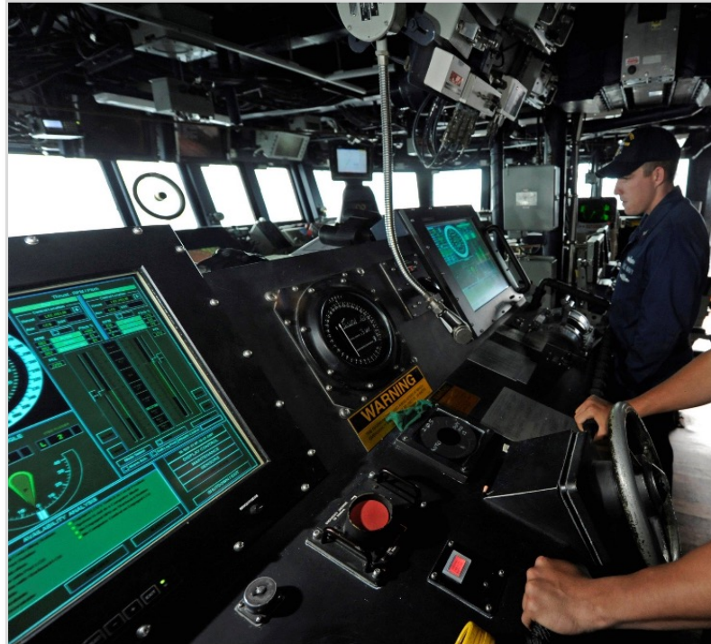
IBNS helm controls on USS Dewey (DDG-105). US Navy Photo
