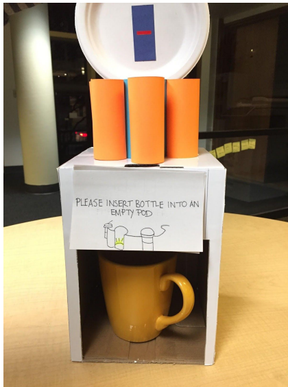
Figure 1.13: The system prompts the user to insert the pill bottle into an empty pod. All empty pods flash to indicate availability.
