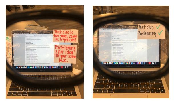
When an individual initially puts the glasses on, the glasses scan the device screen in front of them and let the individual know (via AR technology) if the text size is too small. Similarly, the glasses check if the individual has the ideal positioning relative to the device they are sitting in front of. If both checks are passed, the AR technology displays a pop-up letting the individual know that the text size and positioning are best in terms of reducing digital eye strain symptoms.
