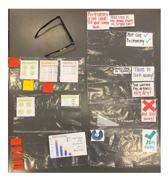
Our prototype includes a pair of glasses frames that will be used to simulate the AR glasses, as well as the various "digital elements" individuals will see while wearing the glasses. We use transparent zip lock bags to simulate the AR technology.
