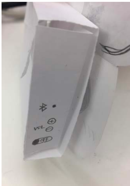
(Figure 1.2) Left side view of panda contains Bluetooth indicator light (green for on and red for off), volume controls, and power switch.
