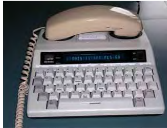
1990s TTY with built-in acoustic modem
