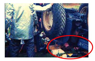
Older tractors with narrow front ends are easily upset
