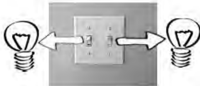
Removing the cover plate, then removing and swapping the switches.
