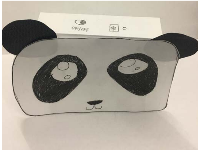
(Figure 1.1) Hardware overview. Kinect-like trackers are located in the eyes of a user-friendly panda.
