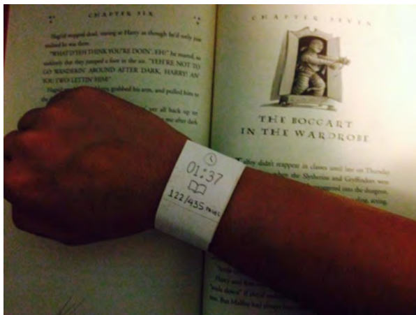
The participant puts on the bookmark which begins timing and tracking the reading session. The participant then reads as normal.
