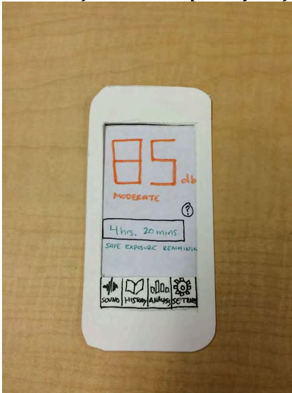
1.a – default screen. User is in moderately loud environment. Essential soundscape details are displayed. (Decibel information will be live updating)
