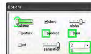
Figure 1: These phosphor widgets use green afterglow effects to show how they have changed. The slider labeled "volume" was dragged all the way to the left. Two of the checkboxes in the next row were unchecked. The combo box was set from 1 to 2.
