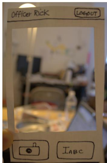
**Figure 7.** *The officer is provided with a camera to take photos of license plate. The prototype has a cutout to simulate the live camera.*
