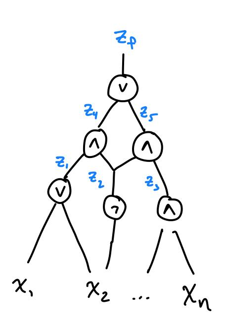
Assign a variable for the intermediate "wires".
