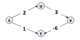
Dijkstra begins with  $S = \{s\}$  and d(s) = 0. Next step would add t to s at distance 1, though actual minimum distance from s to t is -1.
