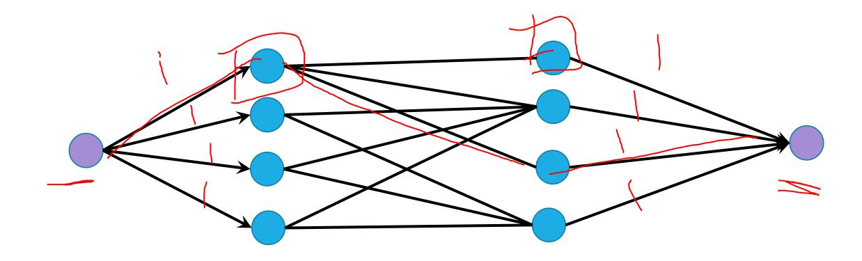
Add a dummy source and sink. Attach each to one side.
