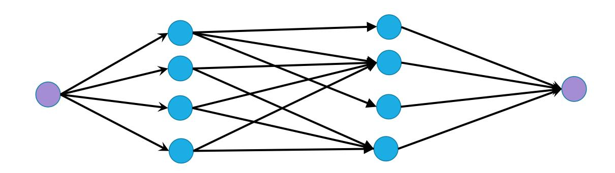
Add a dummy source and sink. Attach each to one side.
