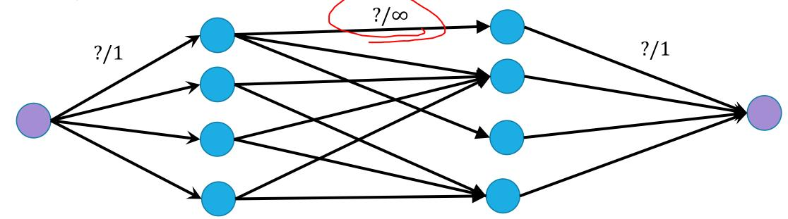
Add a dummy source and sink. Attach each to one side.
