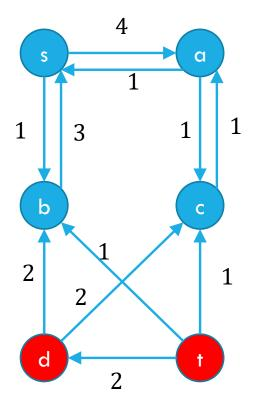
Min cut:  $(\{s,a,b,c\},\{d,t\})$ Edges (b,d),(c,t),(b,t) contribute capacities 2+1+1=4(d,c) doesn't count! Notice it's not used in flow.
