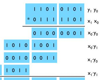
$$T(n) = \underbrace{4T(n/2)}_{\text{recursive calls}} + \underbrace{\Theta(n)}_{\text{add, shift}} \Rightarrow T(n) = \Theta(n^2)$$
