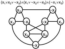
Given 3-CNF formula w, build Independent Set instance y = f(w) as above, run the fast IS alg on y; say "YES, w is satisfiable" iff IS alg says "YES, y has a Independent Set of the given size"
