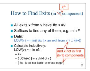
SCC Algorithm #v = DFS number v.low = LOW(v) v.scc = component # SCC(v) #v = vertex\_number++; v.low = #v; push(v) for all edges (v,w) if #w == 0 then SCC(w); v.low = min(v.low, w.low) // tree edge else if #w < #v && w.scc == 0 then v.low = min(v.low, #w) // cross- or back-edge // v is root of new scc if #v == v.low then scc#++; repeat w = pop(); w.scc = scc#; // mark SCC members until w==v
