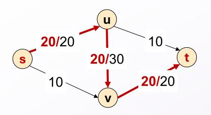
To get more flow from **s** to **t** we need to reduce the flow from **u** to **v**
