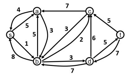
b) On the diagram below, indicate the new flow values for every edge resulting from augmenting f along the path s, a, b, d, t. (Blanks for all edges should be filled in.)
