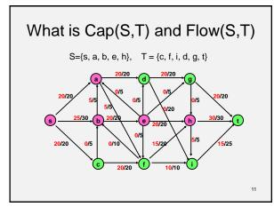
What is Cap(S,T) and Flow(S,T)  $S=\{s, a, b, e, h\}, T=\{c, f, i, d, g, t\}$   $\frac{10/20}{5/5} \frac{20/20}{5/5} \frac{9}{5/5} \frac{20/20}{10/10} \frac{9}{15/25}$  Cap(S,T) = 95, Flow(S,T) = 80 - 15 = 65
