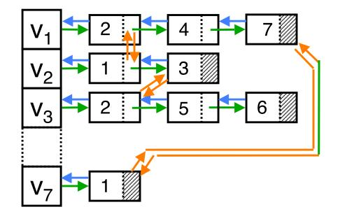
Back- and cross pointers more work to build, but allow easier traversal and deletion of edges, *if needed*, (don't bother if not)
