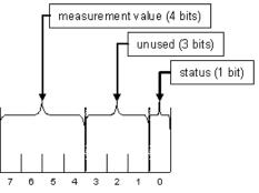
a. How many different measurement values can be reported by this device using this format?
