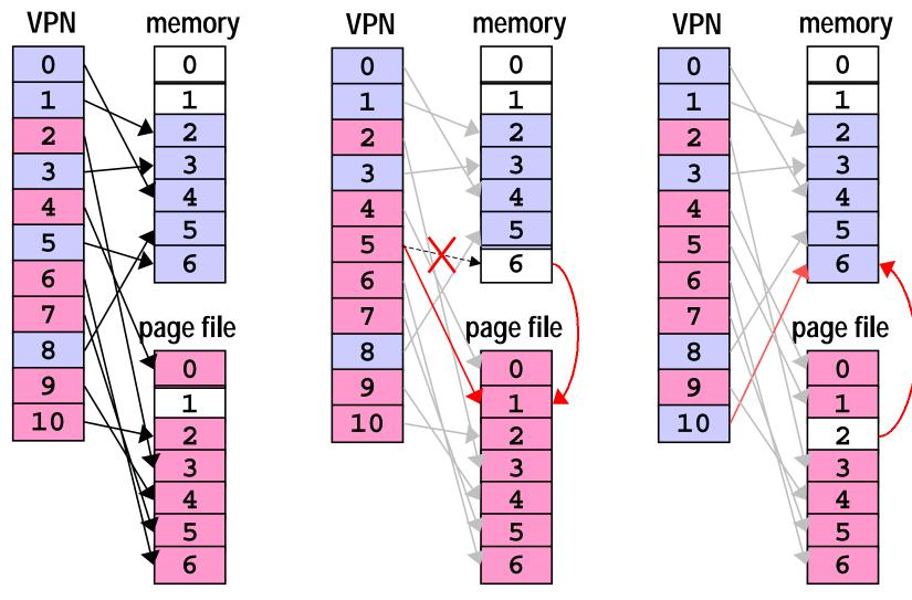
Reference to **VPN 10** causes a **page fault** because it is not in memory.
