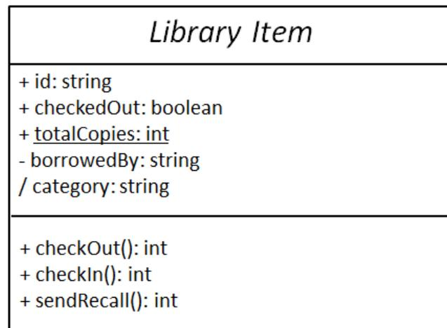
Figure 1: A simple class diagram
