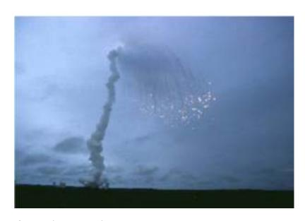
The rocket self-destructed 37 seconds after launch Reason: A control software bug that went undetected
