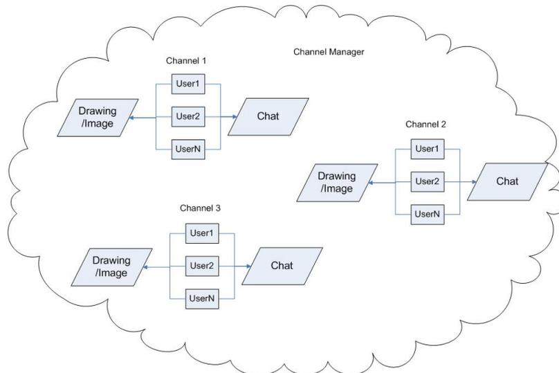
The architecture can be divided into two modules: a channel and a channel manager. The channel's functionality should be to coordinate activity between individual users and to manage the text pane and the drawing area. The channel manager's functionality should be to coordinate each groups activity.
