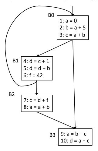
Each of the assignment statements in this flow graph defines a variable like b = 0. Each assignment statement is preceded by a number since we will be interested in a dataflow problem to discover which assignment statements reach other points in the program (precise description below). So, for instance, in the first block, the entry 2: b = a+5 means that the assignment b = a+5 is assignment statement number 2 in the program. Each assignment statement in the entire program has a unique number.
