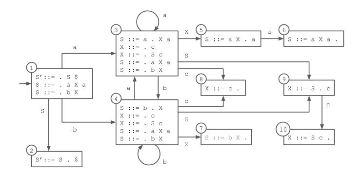
b. Based on your state machine, build the corresponding LR(0) parse table. Start by filling in the ACTION and GOTO headers with the grammar's terminals and non-terminals, respectively, then give each state in your state machine a number and use it to fill out one row of the table.
